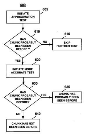
Figure 6 depicts an "approximation test" at step 605 and a "more accurate test" at step 620. The approximation test determines whether the data in the window has "probably been seen before," and may be "performed by computing a rolling checksum of the data and looking up the computed value in a hash table." *Id.* ¶¶ 42, 60–61. The more accurate test may involve "computing a cryptographic hash of the data in the window and looking up the computed value in a hash table." *Id.* ¶¶ 42, 62.
