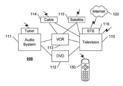
In Figure 1, system 100 includes television 110, audio system 111, DVD player 112, VCR 113, cable interface 114, satellite receiver 115, and set-top box 116. Ex. 1005 ¶ 17. Remote control device 150 provides for
