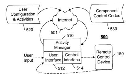
As shown in Figure 5, Dubil's activity manager 510 receives user input, via a user interface 512, and provides control codes to a remote control device 150 via control interface 514. *Id.*  $\P$  30. The database disclosed in paragraph 30 may be distributed among a variety of storage devices and storage systems. *Id.*
