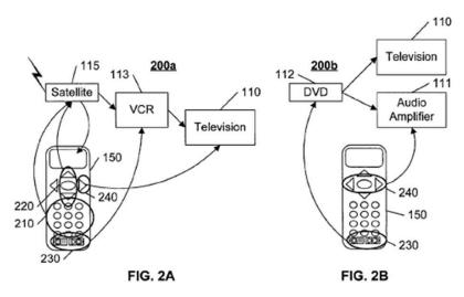
Figure 2A illustrates an activity set 200a for satellite broadcasts.
